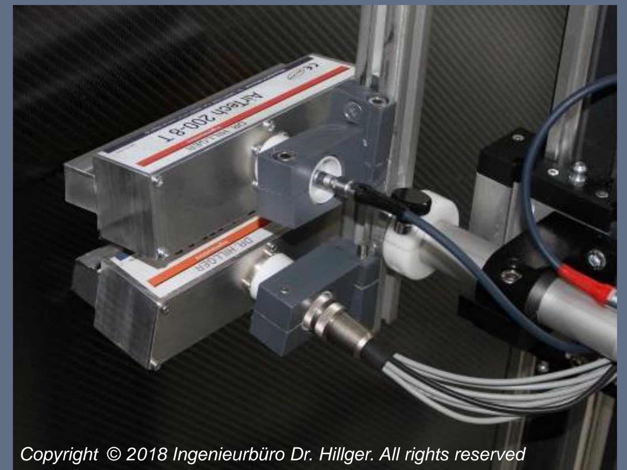
Fig. 2: One-sided investigation with V-arrangement of the probe arrays
