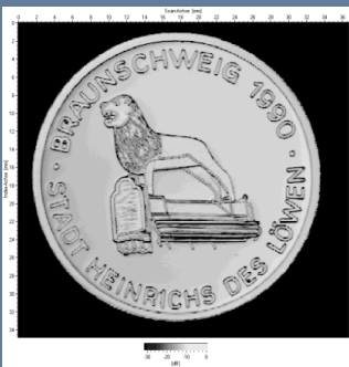
C-scan of a coin recorded with a test frequency of 80 Mhz
