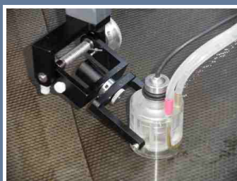
Cardanic fixed transducer adapter with built-in focused immersion transducer
